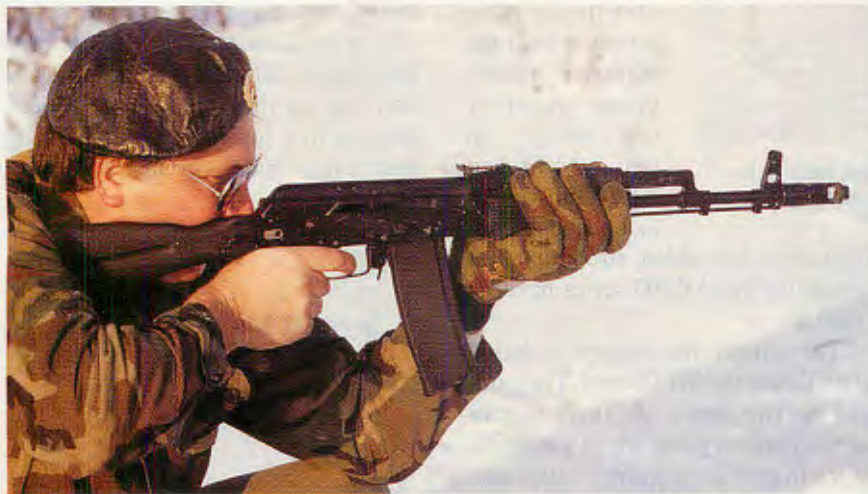
AK101, chambered for the 5.56x45mm NATO round, exhibited significantly greater accuracy potential than rifles in this series chambered for either the 7.62x39mm or 5.45x39mm cartridges.
